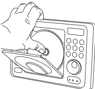
3. Press the **DISC** button and "LOAD" will appear in the display. The disc will automatically start playing.
